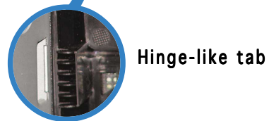
4 Swing the left edge of the front panel outward, then unhook the hinge-like tabs from the holes on the right side of the front panel.
